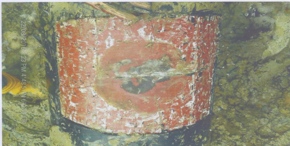
Figure 2.1. 250mm long hacksaw cut with dent
